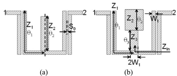
Fig. 1. (a) Dual-mode resonator (b) Stepped-impedance resonator.
