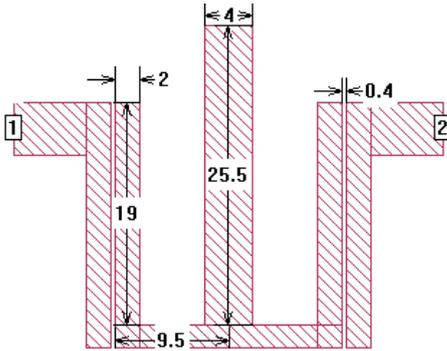
Fig. 3. Layout and dimensions of designed filter in millimeters.
