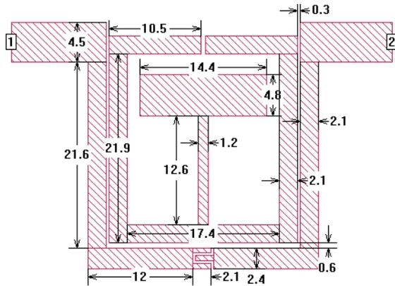
Fig. 5. Dimensions in millimeters of the realized second order filter.
