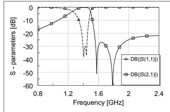
Fig. 6. Simulated  $S$ -Parameters of realized filter.
