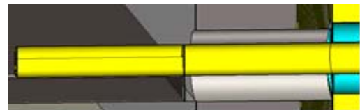
Fig. 10. Detail of microstrip to W-connector transition.
