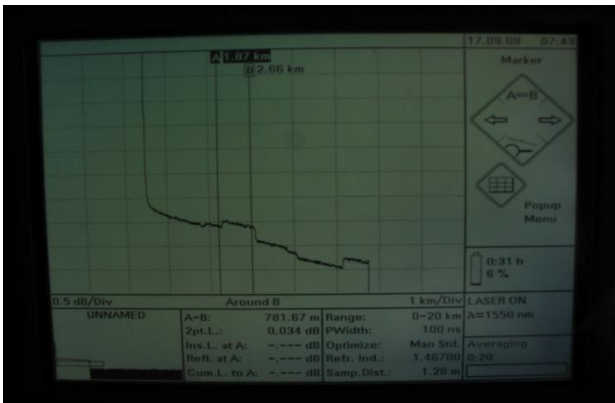
Fig. 3. Measurement of the attenuation between two splices
